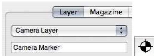
On the Camera Layer, you have to place Markers at the target positions (fitting the original Graphics on the other layer). These Reference Markers have to be present in some way (Crosses, Circles, ...) on the working pieces, also. Usually they are just printed or screen-printed with the first step of manufacturing. At least 3 markers are needed.
